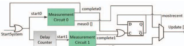
**Figure 4:** Continuous Frequency Measurement Circuit
