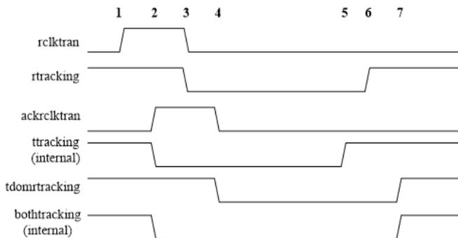
**Figure 7:** Fast Change in Receiver Clock Frequency Timing
