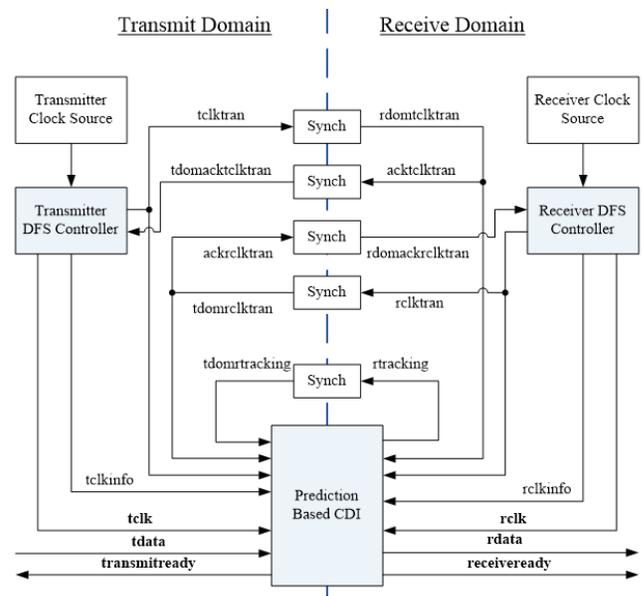
**Figure 6:** High Level Diagram of Fast DVFS Strategy
