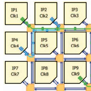
Figure 1: Example of a Multi-Processor GALS System [6]
