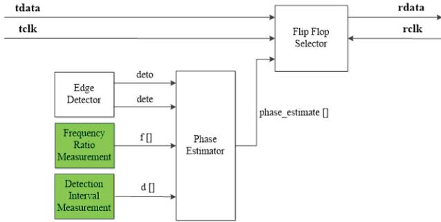
**Figure 2:** Internal EOPS structure
