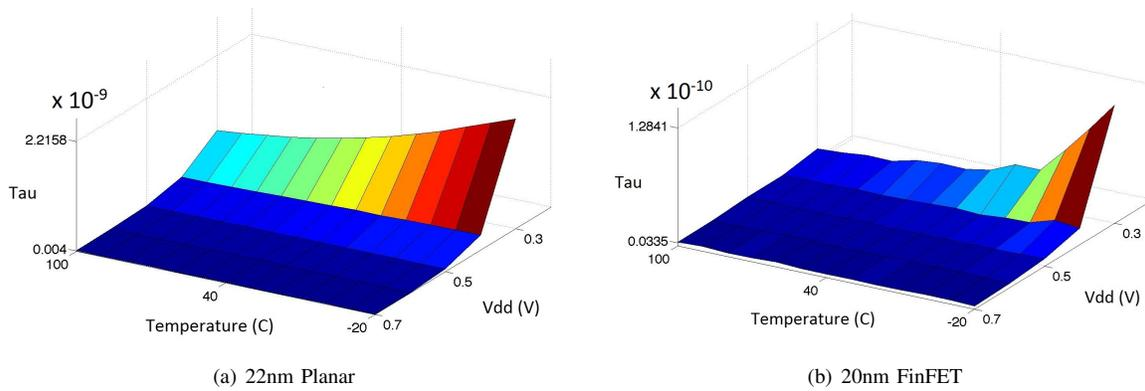
Fig. 6: DLFF  $\tau$  with *Temperature* and  $V_{DD}$  sweep
