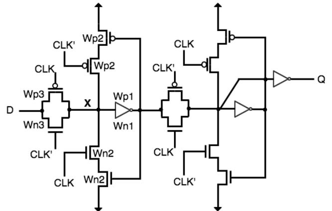
Fig. 4: PowerPC Flip-Flop [11]
