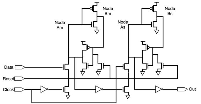
Fig. 3: Dynamic Latch Flip-Flop [9]
