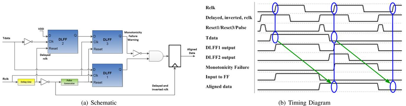
Fig. 10: Robust Dynamic Synchronizer
