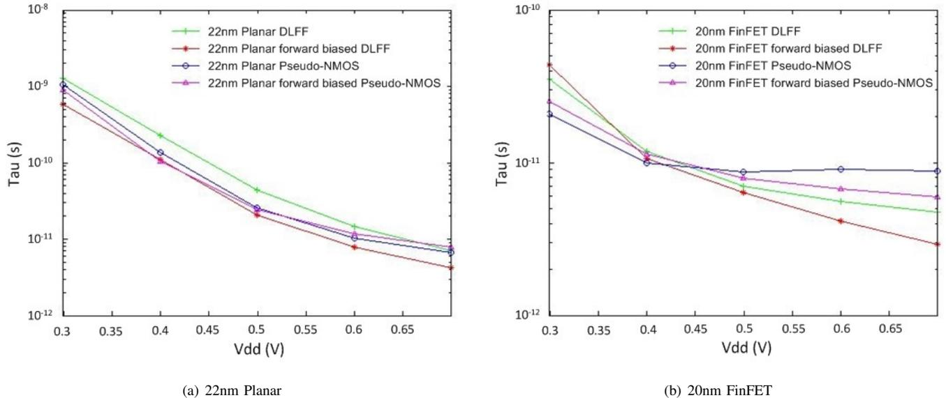
Fig. 8: DLFF and Pseudo-NMOS  $\tau$  when Non-Biased or Forward-Biased with  $V_{DD}$  sweep
