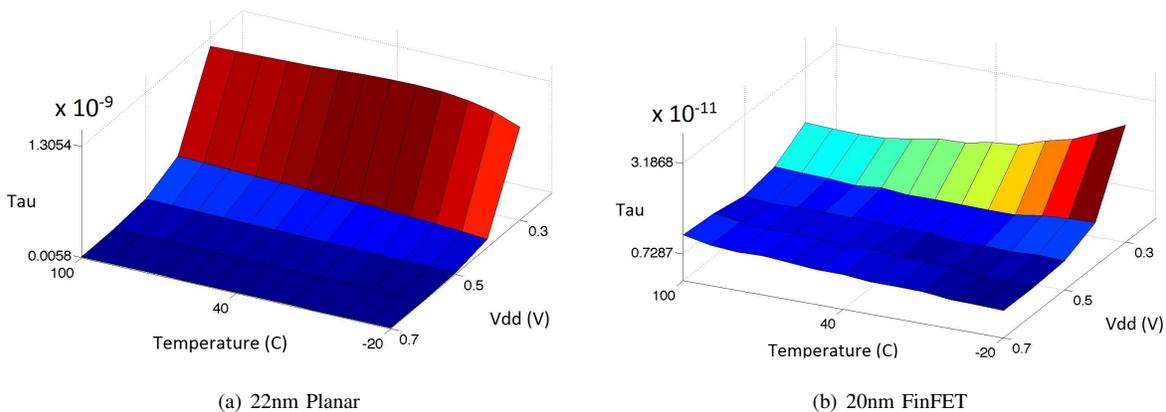
Fig. 7: Pseudo-NMOS  $\tau$  with *Temperature* and  $V_{DD}$  sweep
